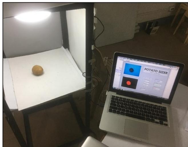
Figure 3. MVS setup
