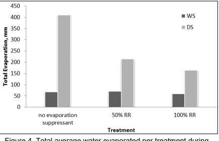
Figure 4. Total average water evaporated per treatment during WS and DS.
