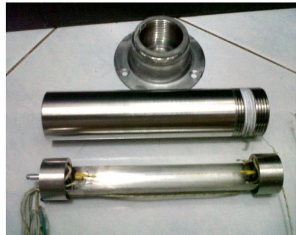
Figure 4. Disassembled hotwire cell.
