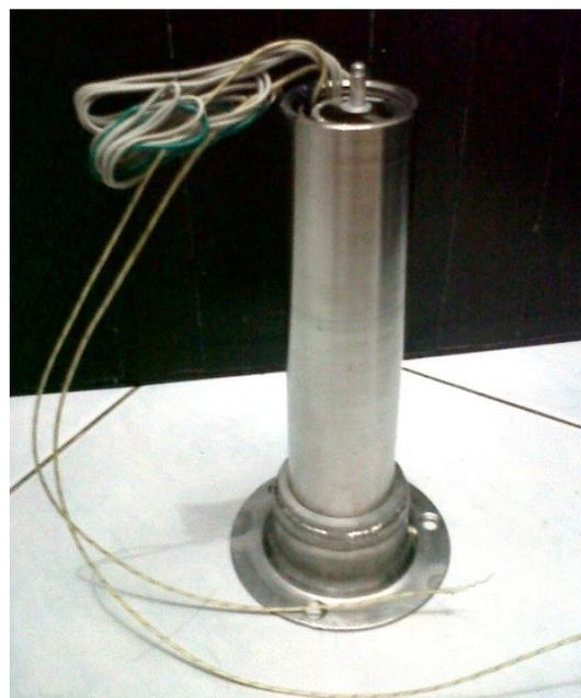
Figure 5. Assembled hotwire cell.
