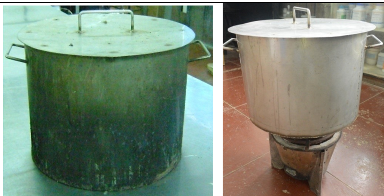
Figure 9. The fabricated stainless cooking vat
